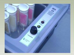
Temperature & status indicators are safe from knocks under the lid, a <u>37</u><sup>0</sup>c Quickset point helps easy initial set up
