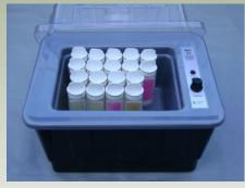
Typical capacity is up to 25 Dipslides or 30 Petri Dishes (95mm)
